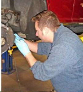
Don Casemore replacing the front disk brake pads
